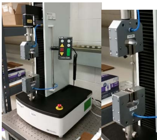
Fig. 8. Photo of the Vantage NX Universal Tester and TA 149 Grips (right inset).
