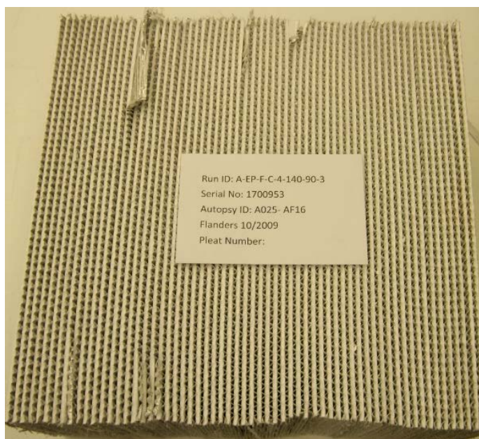
Fig. 6. Photo of the filter pack for test filter A-EP-F-C-4-140-90-3.
