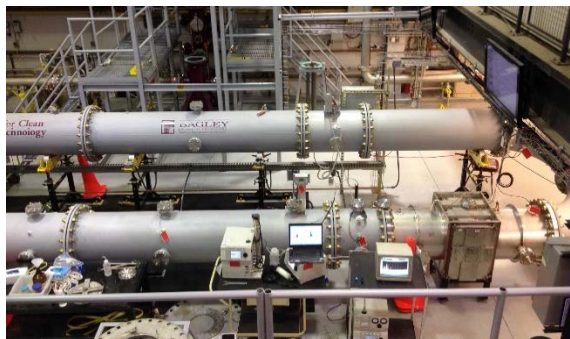
Fig. 2. Photo of the filter housing and aerosol instrumentation of the ALSTS.
